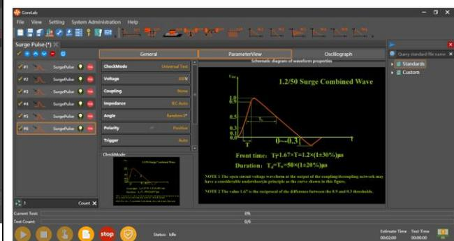
Multiple test step sequences can be added to a test, which is convenient for users to carry out a series of experiments on one or more sets of test objects, and achieve one-click test with simple operation. For test parameters, Corelab also supports scheduling Settings for multiple parameters to achieve iterative testing of parameters, avoiding frequent parameter setting.
